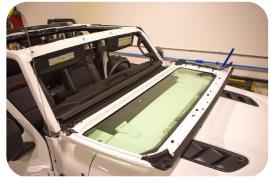
Attach the (4) header clips to the header rail and then reconnect your windshield and wipers.
