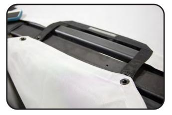
Insert the cord from the bottom up through the bolt hole and then through the bottom front corner of the JK 4D Rear.
