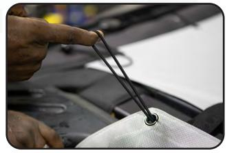
Pull the cord forward to the front seats and back to it's self( be sure these cords are installed on the outside of the 2 JKini straps if using both shades together).
