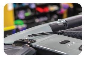
Attach the small spider ball to the square hole of the hard top mounting bracket.
