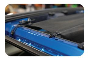
Thread spider ball cord through the bottom of grommet and attach through the top of the left and right footmans loop. Then attach the front hooks to the freedom panel mounting points.
