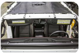
Locate the correct (12) factory T25 screws to remove and add the custom SpiderNubs then replace the (12) factory T25 screws.
