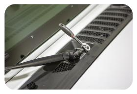
Use the ratchet in the Jeep® toolkit provided to remove the (4) T40 windshield bolts and carefully lower the windshield onto the hood pads.
