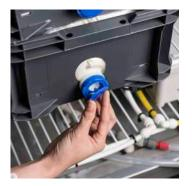
Remove each milk spigot and reseal the bladder connector using the milk suppliers seal. If this still leaks use the ½" bung supplied in your Parts Kit.
