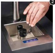
Use the M5 or M6 Alan key supplied with your i-milk and loosen the black load cell connector cap.
