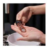
To disassemble gently push the filters and "O" Rings out of the filter housing into a large bowl so as not to lose any parts.
