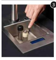
This will expose the loadcell connector rod as shown in the picture showing a Dam in place. Check the dam membrane. If there are any holes replace it with one of the spares in the Parts box.
