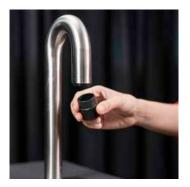
i-milk has a milk filter located on the font outlet. This black fitting delivers a uniform, steady, non-turbulent stream of milk. If the filter mesh becomes blocked it may cause the milk to squirt or froth. To remove the milk filter rotate it as you pull it down.
