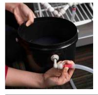
Fill the black cleaning bucket with cold tap water and connect the silicon cleaning line to the bucket.
