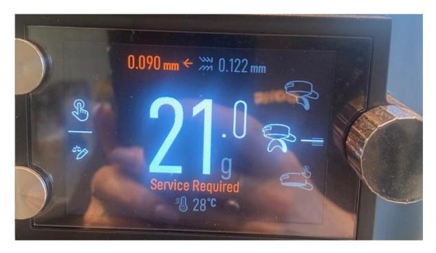
Mahlkonig has advised during the manufacturing programming stage there is potential for the software to glitch causing the burr health counters to prematurely alarm.
