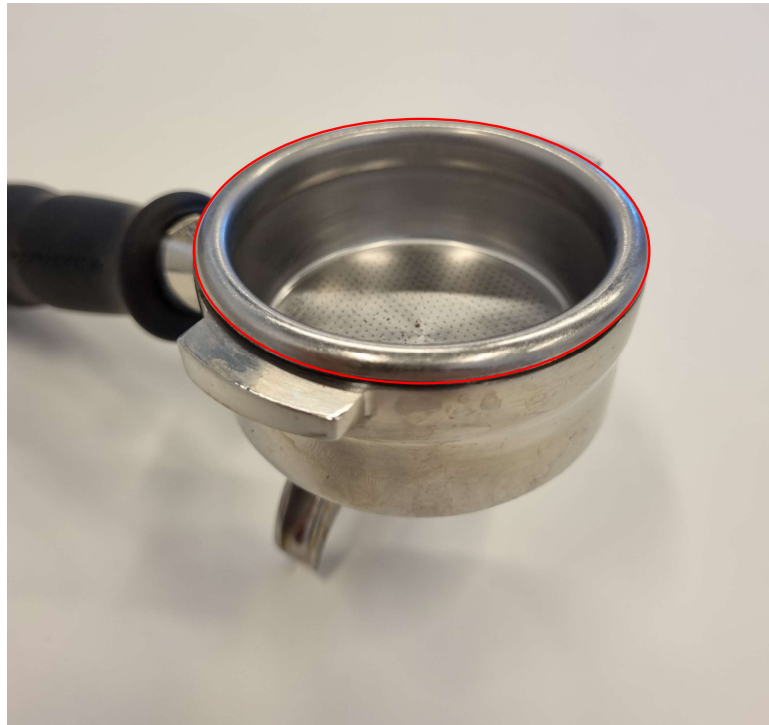
Standard portafilters have the same handle and filter basket outer diameter.
