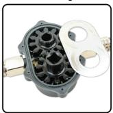
B Clean gears & pump housing.
