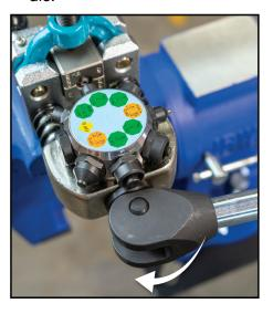
4 Tighten the "T"-handle to clamp down the tubing against the die set.
