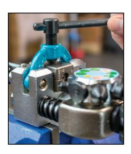
Spin the rotating die head (turret) to OP. 2 and move the lever.
