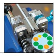
The Flat Faced OP. 0 die is a gauge used to line up the end of the tube flush with the Split Dies. Rotate Die Head so that the flat faced die OP. 0 is facing the end of the tube. Move lever inward toward body using the OP. 0 die as a stop gauge. The tube end must be flush with the end of the die set to create a complete double flare.
