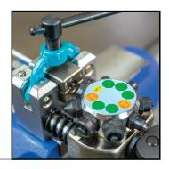
2 Go to OP. 0 to push the tubing flush against the dies.
