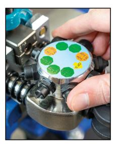
Move lever against tool body exerting sufficient effort to create the inverted portion of the double flare, continuing until it stops.
