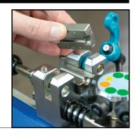
Place the tube between the die halves with the tube end flush with the flared end of the Dies. Rotate clamp back into place, push Clamp Pin through holes and back into the tool until the black knob seats against the body of the tool.
