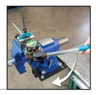
Spin rotating die head with one of the two appropriate sized OP. 2 dies lined up with the end of the tube.
