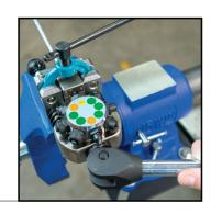
Tighten threaded retainer "T"-handle screw in clamp securely against the die set.
