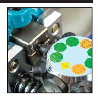
Move lever against tool body exerting sufficient effort to create flare, continuing until it stops
