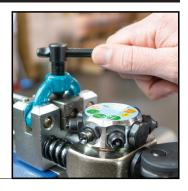
Remove the finished flared tube from the dies.
