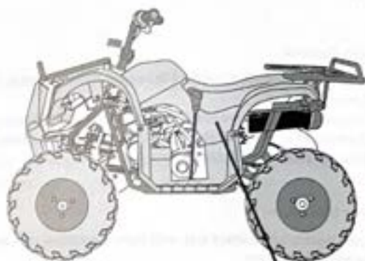
Main Fuse Location
