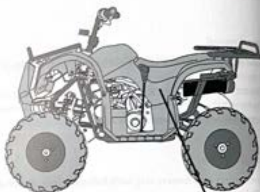
Main Fuse Location
