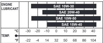
Always use a 4-stroke motor lubricant that meets or exceeds the requirements for API service classification SJ. Check lubricant level before each use.
