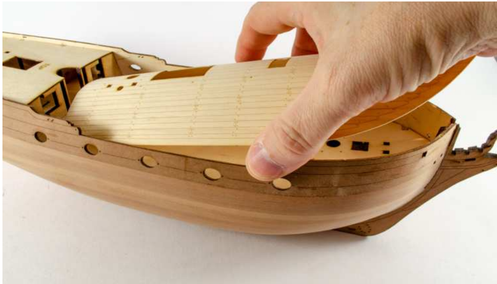
92. Both the Fore and Aft Deck Patterns can now be glued into place. Again, you may need to carefully sand the edges of the Fore Deck Pattern to make sure you get a snug fit. Note how this deck is flexed to allow you to fit it. The decks can be held down with clamps until dry.
