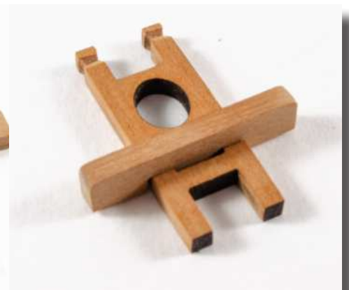
187. Cut the Bowsprit Bitts (54) and Bowsprit Bitts Cross Timber (55) from the 3mm wood sheet and assemble as shown. Also varnish.
