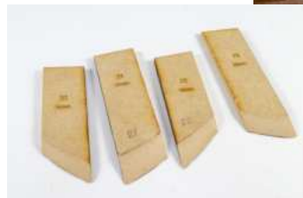
49 (Left). Using sandpaper or a rotary tool, bevel the parts (21 & 22) as shown and then glue them into place on the model.
