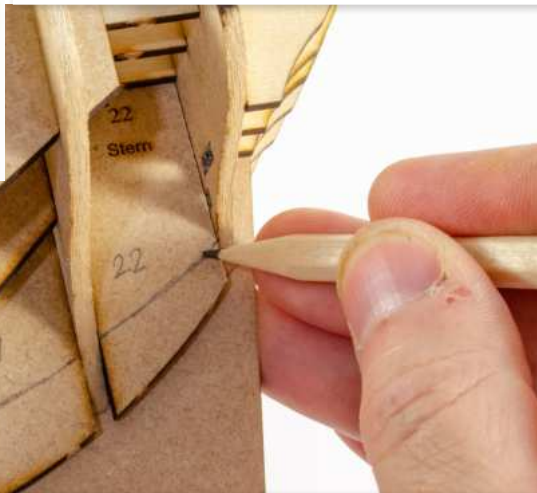
49 (Left). Using sandpaper or a rotary tool, bevel the parts (21 & 22) as shown and then glue them into place on the model.
