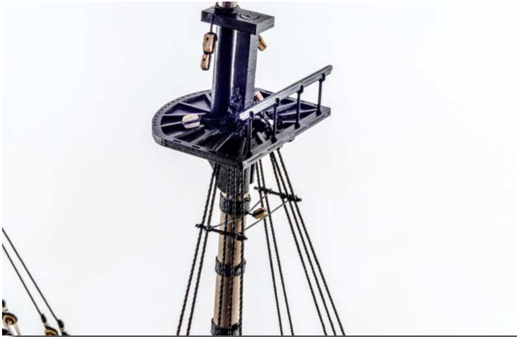
238. With the futtock staves are fitted, you need to add the catharpins as shown here and on the plan sheet #11. These stop the shrouds from deforming/pulling apart, when you add the futtock shrouds. Use 0.5mm black thread for this.
