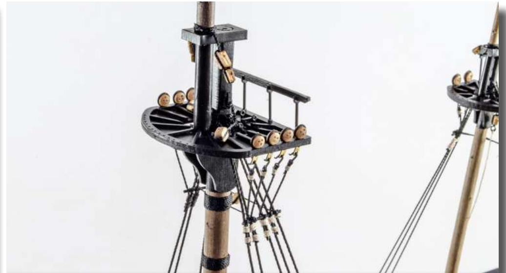
240. After adding the 3mm deadeyes to their 3mm Futtock Strops (PE-93), slide these into position on the lower mast tops. Now take each futtock shroud line and hook into the strops, fastening as shown here and on plan sheet #11. Seize with 0.25mm black thread. Again, I have used natural colour thread to illustrate only.
