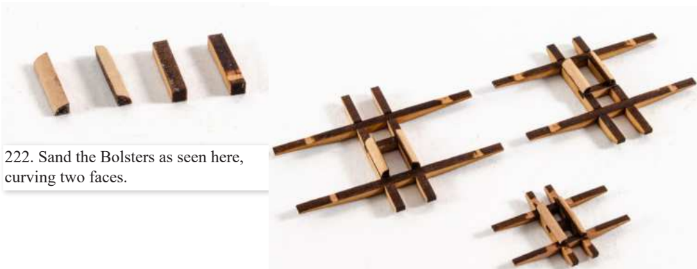
223. Assemble the crosstrees and trestletrees as seen here and on the plans and glue the bolsters into position. Leave to set.
