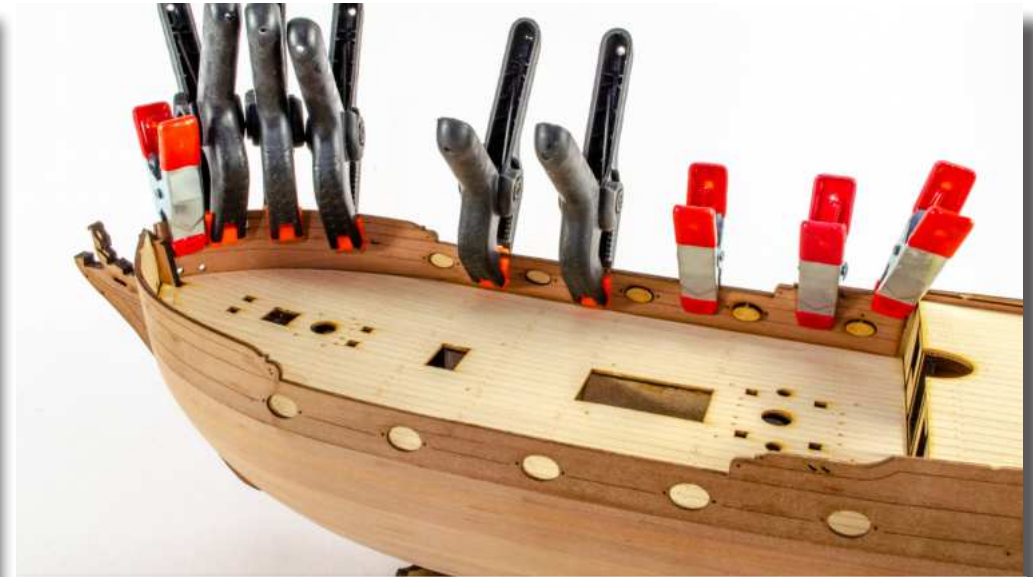
93. Carefully glue the Inner Bulwark Patterns into position and clamp as necessary. We have made these slightly long at the bow side to allow for any hull variations. Make sure that the gun port openings align with the plywood. Use the Oval Side Port Locator Plugs from the 6mm MDF (225) so assist you. These will be removed once the bulwarks are set.
