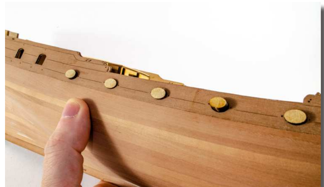
93. Carefully glue the Inner Bulwark Patterns into position and clamp as necessary. We have made these slightly long at the bow side to allow for any hull variations. Make sure that the gun port openings align with the plywood. Use the Oval Side Port Locator Plugs from the 6mm MDF (225) so assist you. These will be removed once the bulwarks are set.
