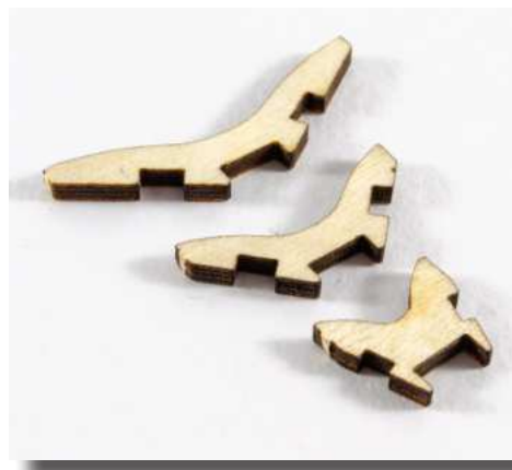
122. Cut the Bow 'V' Frames (33, 34, 35) from the 2mm ply sheet, and file them to shape as shown here. The filing will angle the slots on one side, and also bevel the outer corners. Glue these into place on the prow, as shown. Paint these parts black apart from the surfaces where the rails will fit.
