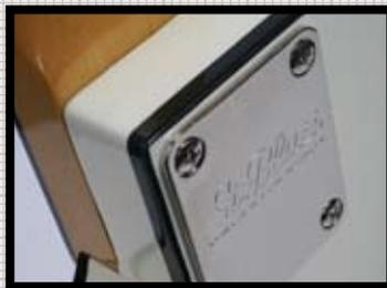
■ Saint Blues has used a traditional bolt-on neck attached to the body by four screws
