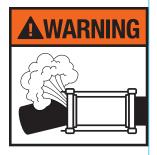
THIS PRODUCT DOES NOT RESTRAIN PIPE MOVEMENT. Proper anchoring is required to prevent pipe pullout. Failure to anchor or improper anchoring can result in dangerous pipe content escape, property damage, serious injury, or death. Read the product installation instructions prior to installing this product.
