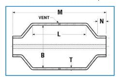
Built to rigid Dresser specifications, Style 220 sleeves have a minimum yield strength of 50,000 psi and an ultimate strength of 70,000 psi. Style 220 sleeves are supplied in all sizes, lengths and thicknesses as shown in charts. Larger sizes and lengths available upon request.
