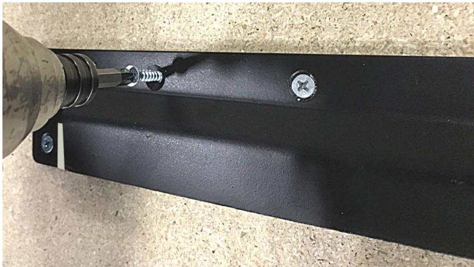
**NOTE:** The pictures at left are a simple representation of the act of attaching the Loose Hook Brackets to the floor.
