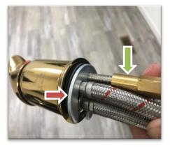
7) Feed the lines of the faucet into the round hole of the bowl. Making sure the round gasket is underneath the faucet.
