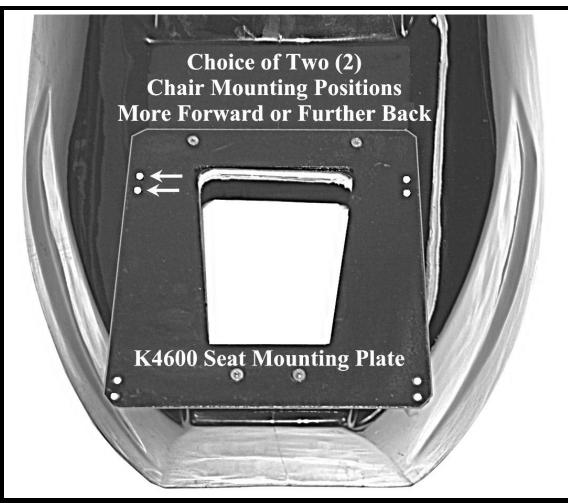
Remove the Seat Mounting Plate and attach it to the bottom of the Chair Seat.
