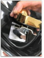
12) Place the Vacuum Breaker Plate on top of the square hole on the bowl with the clamp of the plate place as shown and tighten down.
