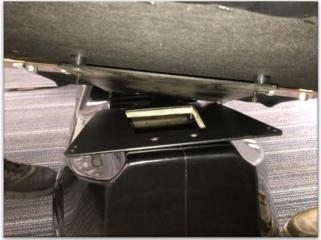
2) Using (1) washer and (1) nut tighten down chair top to the mounting plate. A 10mm wrench (not provided) is needed to tighten down the rear nuts.
