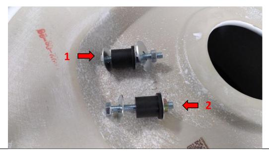
6) Insert the Grommet like so and tighten down in all 3 spots of the bowl.
