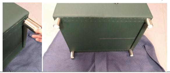
3) Take the shorter leg and screw it down with the wood screws in the center of the base as shown.
