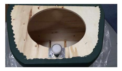
4) On the back of the Chair remove the nuts and washers and attach the Base using the nuts and washers on the inside of the Base.
