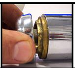
Unscrew the silver crown by turning counter-clockwise.
