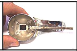
Insert a flat blade screwdriver into the buttonhole (it may take a 2.5mm allen wrench instead). Choose the proper size.
