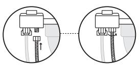
Affix the flexible steel hose from the mega adapter to the cold water port on the underside of the TUSHY console.
