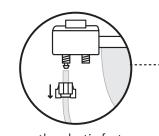
Unscrew the plastic fastener from the hot water port on the underside of the TUSHY console. Thread the other end of the plastic tube through the plastic fastener.
