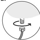
Disconnect the existing flexible hose from your toilet tank by turning it counter clockwise, disconnecting it from the bolt under the tank.
