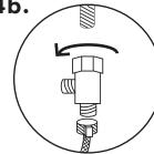
Attach the flexible hose to the bottom of the mega adapter and then screw the top of the mega adapter clockwise onto the tank connection. Be careful not to over-tighten! \*
