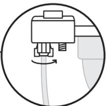
Finally, tighten the plastic fastener clockwise to the hot water port sealing the connection.
