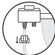
Unscrew the plastic fastener from the hot water port on the underside of the TUSHY console. Thread the other end of the plastic tube through the plastic fastener.
