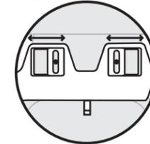
Now for the big moment... place the TUSHY on top of your toilet and line up the sliding seat fasteners with the holes in between the bowl and the tank used for mounting the toilet seat.
