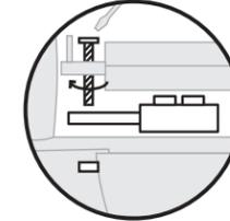
Reattach the toilet seat on top of the TUSHY by threading the toilet seat bolts through the sliding seat fasteners and through the toilet's mounting holes. Fasten the bolts by turning them clockwise.
