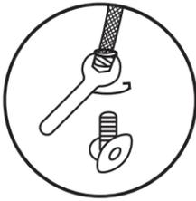
Disconnect the existing flexible steel hose from the warm water supply valve by turning it counter clockwise.
