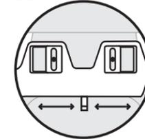
Make sure the nozzle is lined up in the center of the back and not too close to the edge of the bowl to allow room for it to be adjusted in use.
