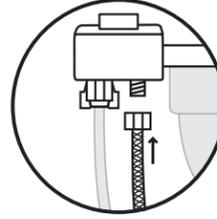
Affix the flexible steel hose from the mega adapter to the cold water port on the underside of the TUSHY console.
