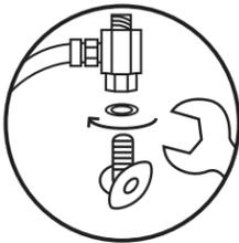
Place the rubber washer inside the mini adapter. Fasten the mini adapter to the warm water supply valve by turning clockwise first using your hand and then using a wrench. Make sure it's tight, but don't go nuts. \*\*\*
