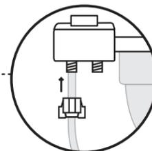
Next, place or twist the plastic tube onto the hot water port under your TUSHY. (If needed, you can soften the end of the tube with hot water or a hair dryer.)
