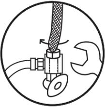
Reconnect the warm water hose to the top of the mini adapter by turning clockwise using your hand and then using a wrench. Again, make sure it's tight, but don't go nuts.
