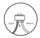
WARM WATER CONNECTION: Thread the other end of the plastic tube from the warm water connection through the plastic fastener and onto the labeled port under your TUSHY. Tighten the fastener.
