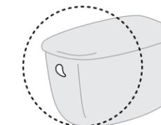
Flush your toilet to drain the tank completely. Hold down that flusher until it empties! (A couple inches of water is okay.)
