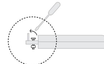
Flip up the screw caps behind the seat with a flat head screwdriver to access the screws. You may need to hold the bolt beneath the screw with your other hand while unscrewing. Remove the seat and set aside. Dealing with a unique toilet seat? Check out HelloTushy.com/hacks for some tips.
