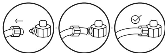
Unscrew the metal fastener from the mini adapter. Grab the plastic tube and thread one end of the tube through the fastener, then onto the mini adapter port and tighten the fastener to secure the connection. \*
