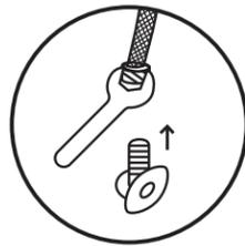
Disconnect the existing flexible steel hose from the warm water supply valve with a wrench. (If you have a hard metal pipe, visit [HELLOTUSHY.COM/PARTS](https://www.hellotushy.com/parts) to get a flexible hose.)
