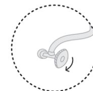
Turn off the water valve near the toilet and the warm water supply under the sink in small increments to avoid damage, especially to older valves. There may be some mineral build up - slow and steady wins the race. Try twisting it in one direction and then the other, each time rotating a little further until it's free to turn all the way around.
