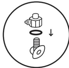
Place the rubber washer in the mini adapter. Fasten the mini-adapter to the warm water supply valve using your hand. Make sure it's tight, but don't go nuts.
