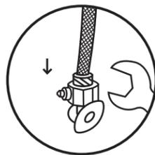
Reconnect the flexible steel hose to the other side of the mini adapter using a wrench.
