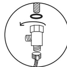
Place the rubber washer in the mega adapter. Screw the adapter onto the tank connection and then attach the flexible hose to the bottom of the adapter. Do not over tighten. **Optional:** Use teflon tape inside each connection. \*\*
