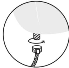
Disconnect the existing flexible hose from your toilet tank. To unscrew the connection, turn right. (If you have a hard pipe, visit [HELLOTUSHY.COM/PARTS](https://www.hellotushy.com/parts) to get a flexible hose.)
