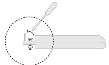
Flip up the screw caps behind the seat with a flat head screwdriver to access the screws. You may need to hold the bolt beneath the screw with your other hand while unscrewing. Remove the seat and set aside. Dealing with a unique toilet seat? Check out [HELLOTUSHY.COM/HACKS](https://www.hellotushy.com/hacks) for some tips.
