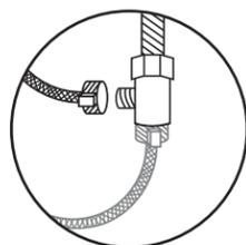
Attach the flexible hose to the adapter for connection to your Tushy. Use a wrench to tighten it if necessary. \*\*
