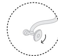
Turn off the water valve near the toilet in small increments to avoid damage, especially to older valves. There may be some mineral build up - slow and steady wins the race. Try twisting it in one direction and then the other, each time rotating a little further until it's free to turn all the way around.
