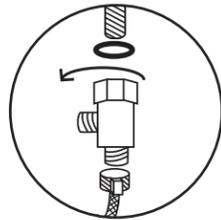
Place the rubber washer in the adapter. Screw the adapter onto the tank connection and then attach the flexible hose to the bottom of the adapter. Do not over tighten. **Optional:** Use teflon tape inside each connection. \*
