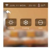
Note: Enter the password "168" in "Parameter" and set the heating & cooling type by modifying NO2.
