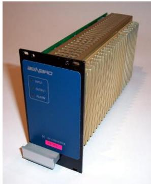
The equipment is protected against input reverse polarity by a diode across the input, which causes an internal fuse to trip.
