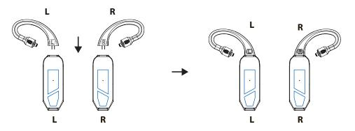
**Ear loops connected to the GO pod Max touch control units** Two ear loop pairs are supplied: 0.78mm 2-pin, MMCX.
