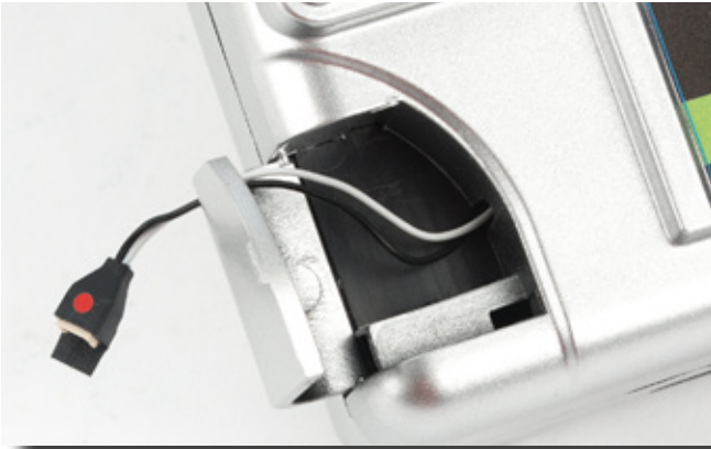
Open door on lower left of transmitter
