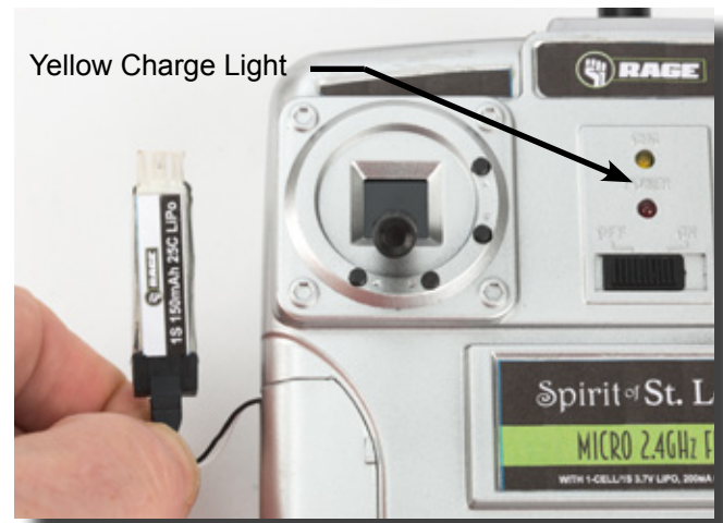
The yellow charge light on the transmitter lights during charging. When the light goes out, charging is complete.
