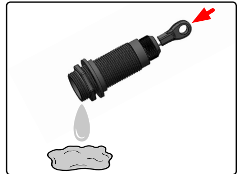
Drain the oil from the shock absorber.
