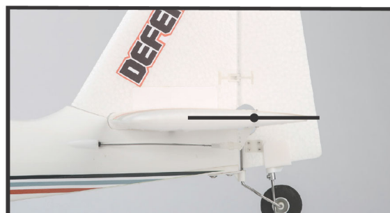
Elevator properly centered.
