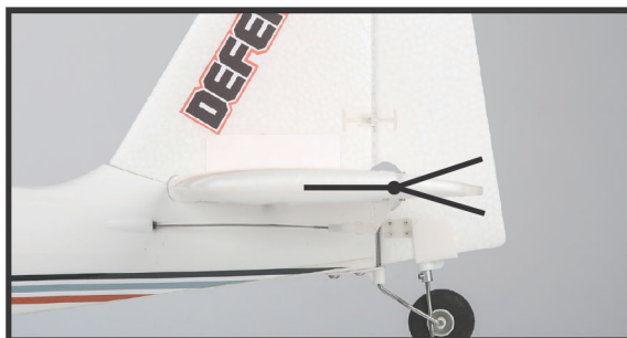
Elevator not properly centered.
