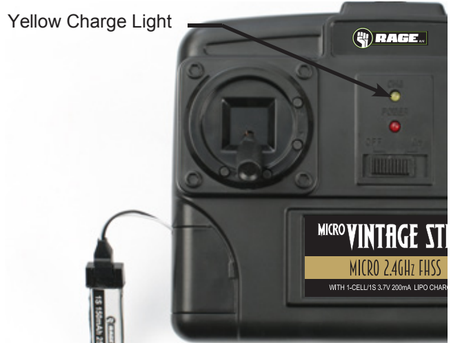
The yellow charge light on the transmitter lights during charging. When the light goes out, charging is complete.
