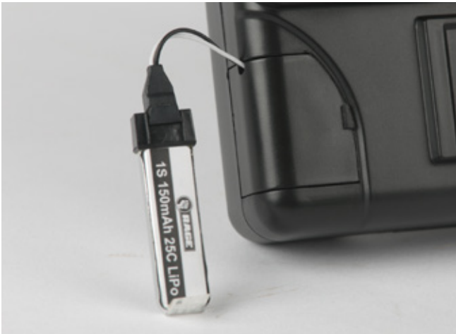
Plug flight battery into charge plug. Make sure to maintain correct polarity by aligning the red dots when plugging in the battery.
