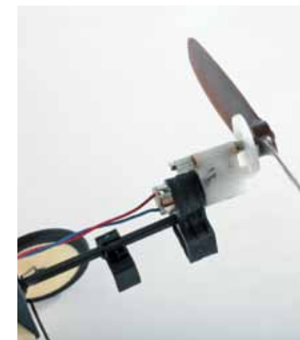
Right: The motor is brushed and comes attached to a gear drive to spin the propeller.
