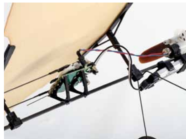
Located below the wing, the airborne control board combines receiver, speed control, and servo functions.
