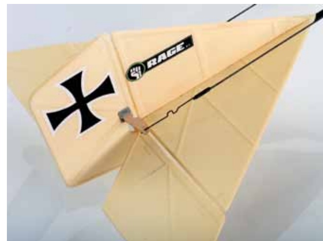
Left: The tail surfaces, control linkage, and wire tailskid all come installed.
