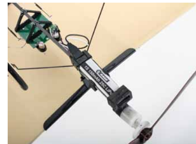
Just in front of the wing and below the motor is a holder for the LiPo flight battery.
