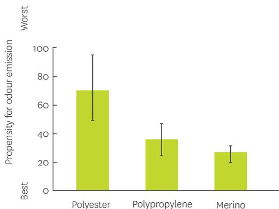
Figure 2 above displays the Propensity for odour emission, and the maximum and minimum scores, (depicted by the black lines).
