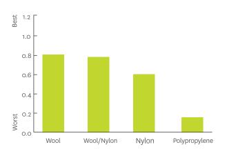
Figure 2. Energy (Radiant Panel Test) required to ignite carpets (Source: Wools of New Zealand)
