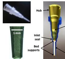
AssayMAP utilizes disposable cartridges containing a 5 µL packed bed with any resin (particle size 20 – 100 µm). The bed is retained by insert-molded bed support filters. Above the bed is an inlet seal and hub (used for robotic operation) and a sample cup (which can hold up to 200 µL).
