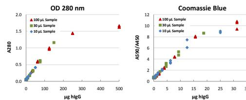
The same data are shown below plotted vs. hlgG concentration in µg/mL. If the full range of sample volumes and the two readout methods are utilized, the assay has an effective range of 10 – 10,000 µg/mL.
