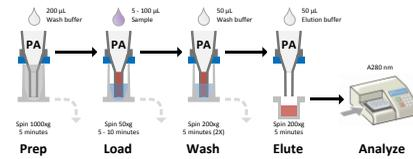
Readout of the plate is performed in a conventional plate reader. First the plates are read at 280 nm. Optionally a colorimetric protein assay reagent (such as Coomassie Blue) can be added for increased sensitivity and read at visible wavelengths (e.g. 590 and 450 nm).
