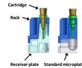
In operation, cartridges are loaded into racks stacked on the appropriate plates, and sample, buffers and other reagents are pipetted into the cartridge cups. The cartridge/rack/plate is then spun in a standard microplate centrifuge to drive the liquid through the bed. With a 2-plate rotor, up to 192 samples can be processed simultaneously (up to 384 with a 4-plate rotor). Fewer samples can be processed by loading fewer cartridges in the rack.
