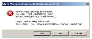
**A.** Ensure that the cartridge is installed correctly as per section 3.6.2, above.
