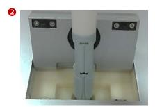
Note: Cartridges can only be inserted in one orientation as shown in figure above.
