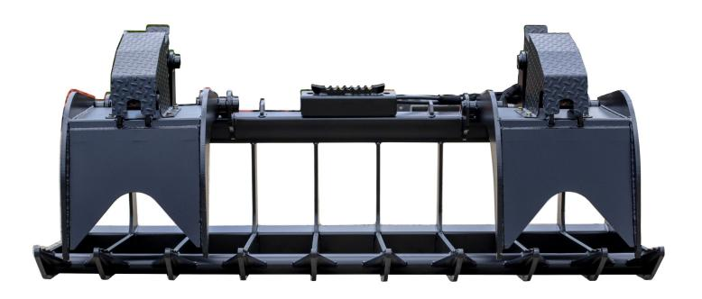
5/8 inch A-36 steel construction with counter-sunk grease pins and bushings at all hinge points. Diamond plate cylinder and rod covers.
