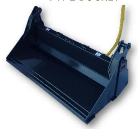
The 4-N-1 Bucket attachment is versatile yet durable for your skid steer jobs. Our 4-N-1 is ideal for grappling, dozing, back-filling, loading, digging and fine grading. The protected cylinders are 2.5" x 8" stroke on the Heavy Duty Buckets and are 3" x 8" stroke on the Extreme Buckets. The Heavy Duty Buckets come with a  $\frac{1}{2}$ " x 6" and  $\frac{1}{2}$ " x 4" cutting edges at ground points. The Extreme Buckets come with  $\frac{1}{2}$ " x 6" cutting edges at all ground points.
