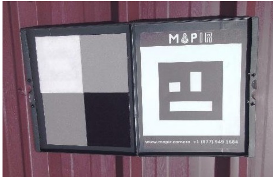
Figure 1: The calibration target.
