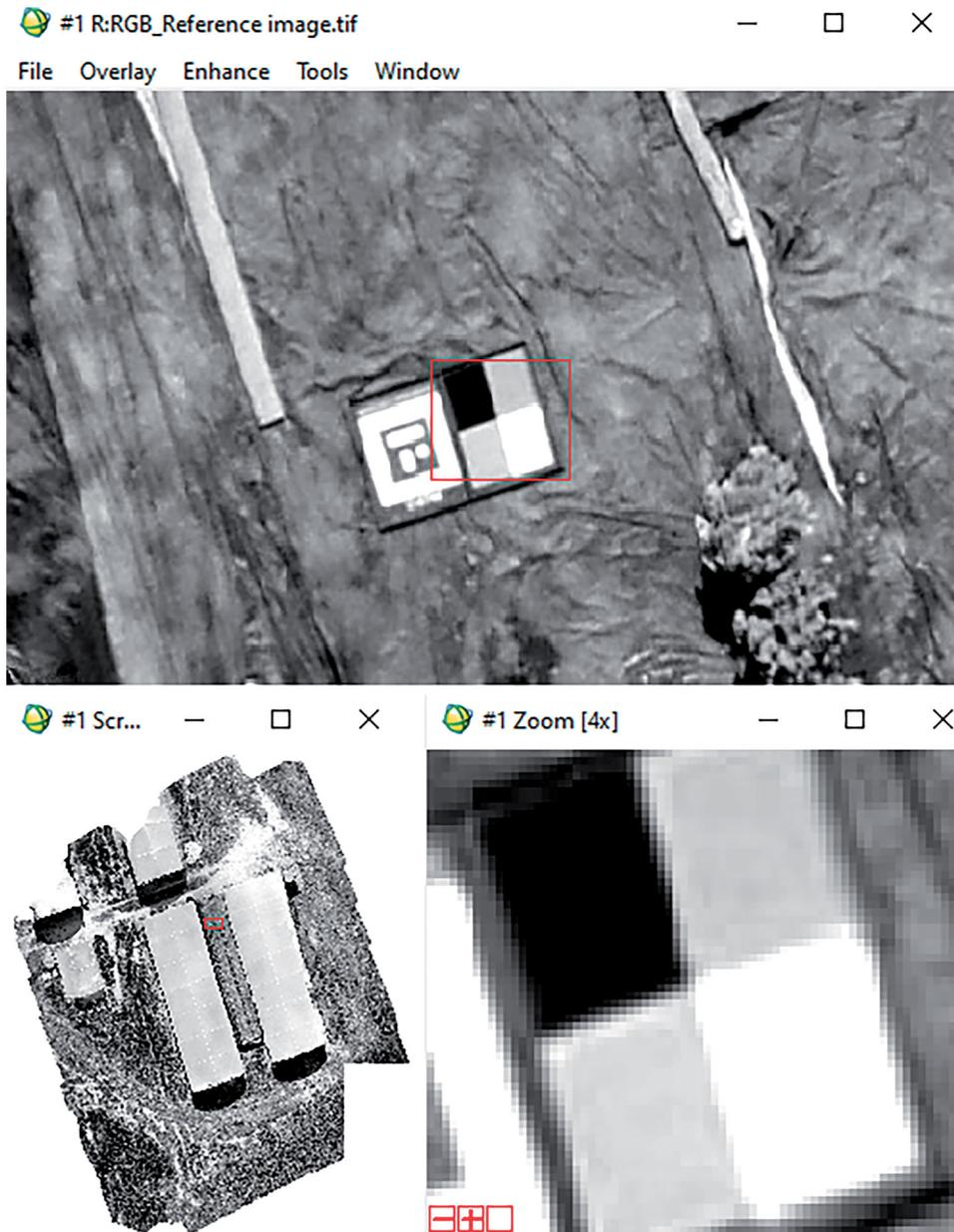
**Figure 2.** Calibration target of the Mapiir Survey3W camera to extract the mean values of dark and light pixel sets.
