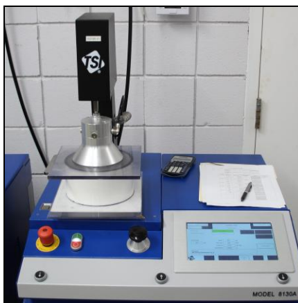
Figure 4: Respirator filter under efficiency test
