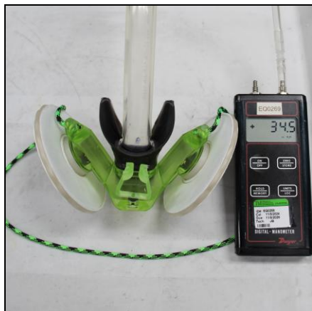
Figure 3: Respirator mounted for resistance measurement
