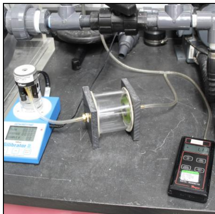
Figure 5: Valve under leakage test.
