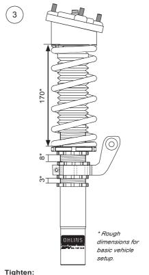
Lower spring seat and lock ring: 50-60 Nm Lock nut M14: 35-40 Nm
