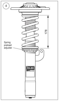
recommended spring preload may vary. Adjust the spring preload until you have reached your desired ride height. Make sure that the spring is always preloaded.
