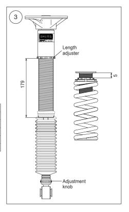
may vary. Adjust the spring preload adjuster until you have reached your desired ride height. Make sure that the spring is always preloaded.
